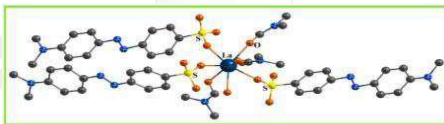
Fig. 1. The molecular structure of ([La(L) 3 (DMF) 3 (H 2 O) 2 ). The hydrogen atoms are omitted for more clarity
